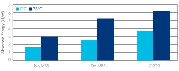
Typical calendering formulation (phr): PVC Kw57: 100, Octyl Organotin Stabilizer: 1.2, internal lubricant: 0.8, ESBO: 1, Plastistrength<sup>®</sup> 550 process aid: 1, Plastistrength<sup>®</sup> 770 process aid: 0.7, Clearstrength<sup>®</sup> C impact modifier: 9
