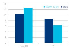
Formulation (phr): PVC Kw62: 100, tin maleate: 2.1, internal lubricant: 0.8, ESBO: 1, Plastistrength® 550 PA: 2, Plastistrength® L1000 PA: 0.15, oxidised PE wax: 0.15, UVA: 0.3
