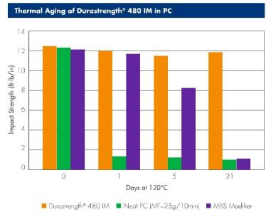
\*ASTM D256 specifications for notched IZOD impact tests. Formulations contain 5% impact modifier
