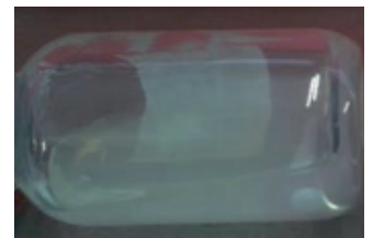
15 wt% of Clearstrength® XT100 into MMA monomer → easy dispersion
